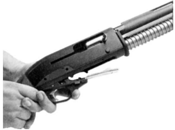
Figure 18. Remove trigger group
