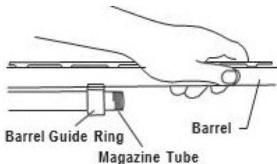
**Figure 2. Shotgun assembly**
